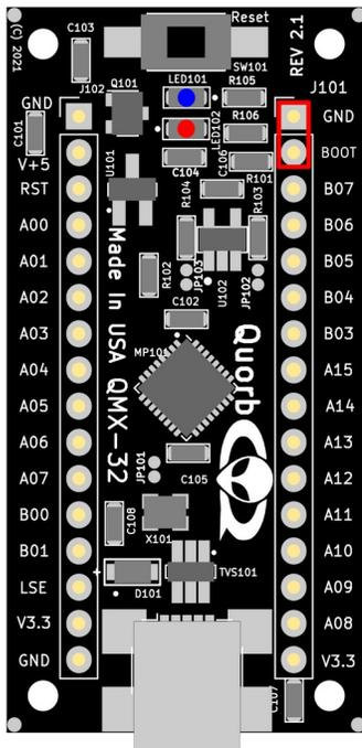
2. Press the reset button. If the red and blue LED are both on, then the board is now in programming mode. Open the STM32 Cube programmer.
