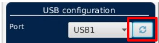
1. Note: If the port selector says 'No DFU detected,' then hit the reset button on the module then refresh, and it should appear.
